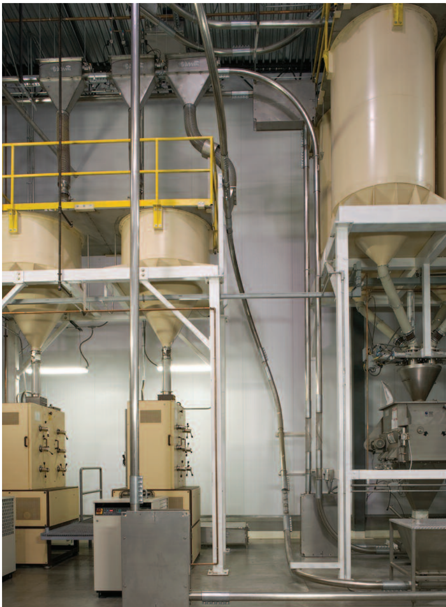
The roasted beans discharge from the holding silos (right) into a conveying system that moves them vertically and then horizontally above the two grinders (bottom left).
