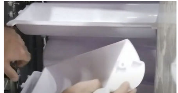
(Manual removal of bucket for cleaning out of place. Removing and replacing the buckets alone could take an hour or more as the conveyor must be jugged to get access to all the buckets)
