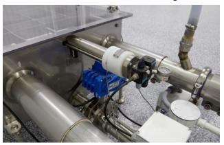
One area of emphasis during service calls to current customers is a retrofit process to replace the existing stainless-steel springs using our pneumatic tensioning system. The pneumatic devices manage cable tension. Proper cable tension is a major contributing factor to the overall function, dependability, longevity, and power of the conveyor system.
