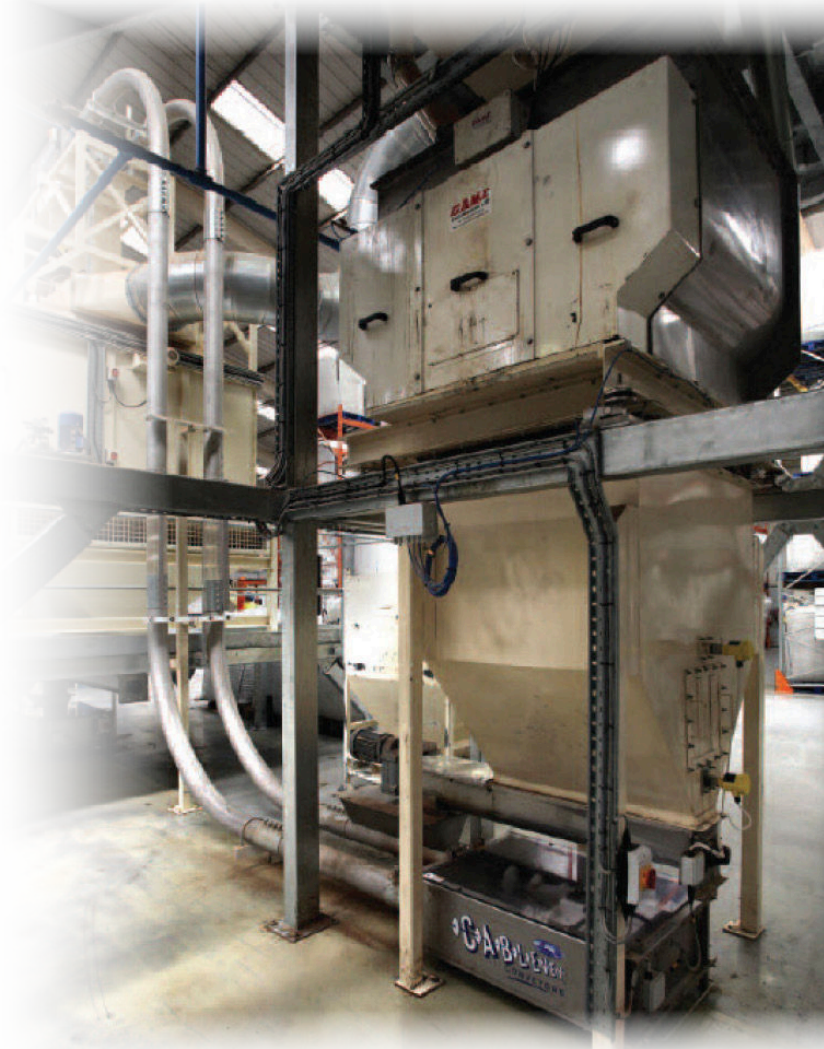
The stainless steel tubular drag cable conveyors provides dust-free conveying from the mixer up to the cooler inlet.
