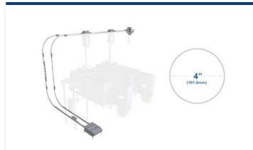
Our **4in diameter conveyors** are our most popular system. They are used to transport products such as flaxseed, whole-bean roasted coffee, or raw peanuts. They are rated to move up to 21,000 lbs/hr of material or approximately 525 ft³/hr.
