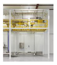
With multiple lines already operating within a finite amount of space, a new or replacement system that can be configured in multiple ways to fit within that space or footprint has heightened importance. Replacing a bucket elevator for example, with a drag cable system, involves careful selection of sweeps and placement of the turnaround, not just for space concerns but also to facilitate cleaning and maintenance.
